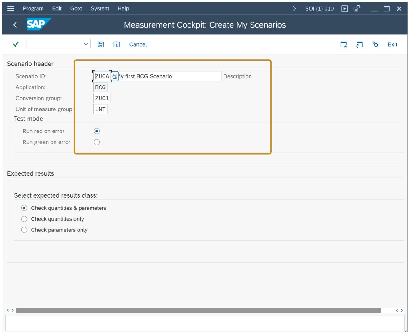
In the details screen, the reading group values are defaulted as input parameters. Now enter the LNG observed temperature as -161.000 °C and the transaction quantity of 100,000.000 M3L. Then select the “Calculate expected result” push button, confirm the calculation and save the scenario (CTRL + F4), confirming all messages:
