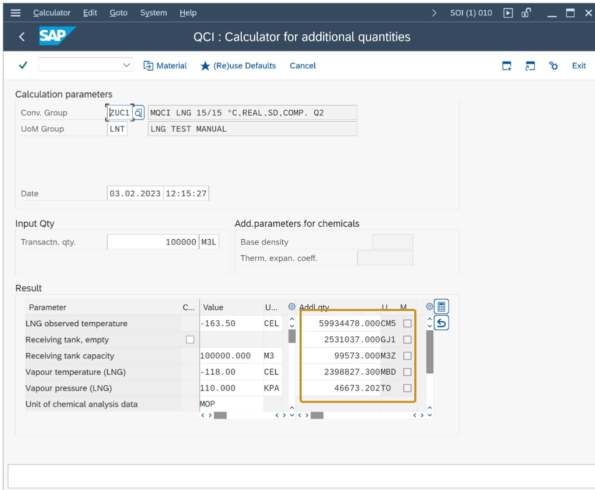
The screenshot shows the SAP QCI Calculator interface. The 'Calculation parameters' section includes 'Conv. Group' (ZUC1) and 'UoM Group' (LNT). The 'Input Qty' section shows 'Transactn. qty.' as 100000 M3L. The 'Result' table is as follows:
