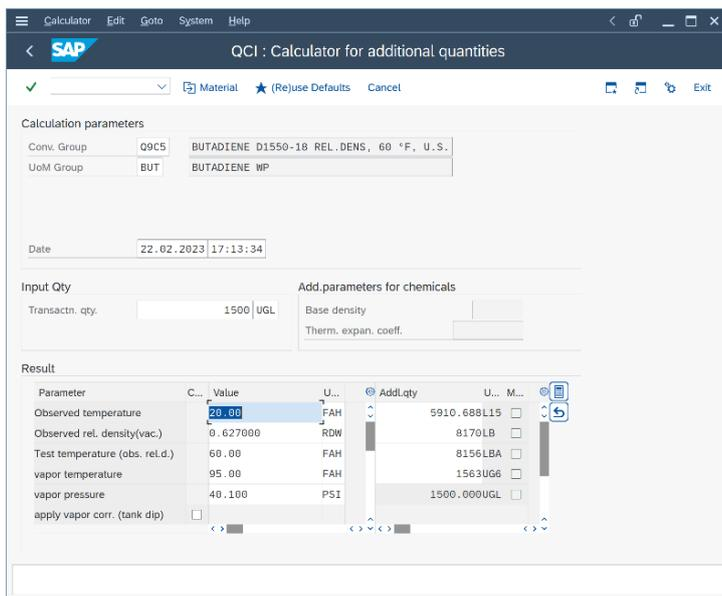
Conversion group X9C5 is a copy of Q9C5, where we simply replace the ASTM D1550 vapor space calculation model function with the generic LPG ideal gas vapor space calculation model function and define the molar mass of Butadiene in the reading group.
