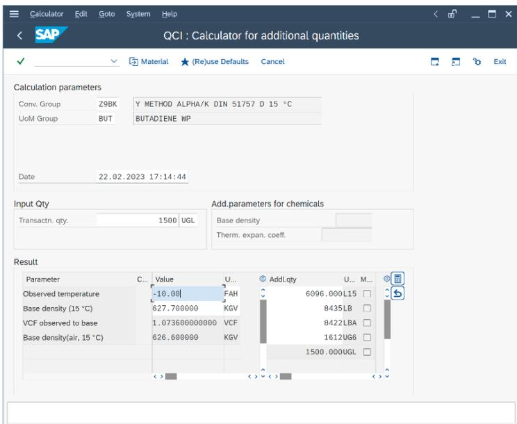
For the comparison calculations of the CTL factor related quantities, we vary the observed liquid volume temperature between -10 °F and 110 °F in 10 °F increments and turn the vapor space calculations off. The following table summarizes the comparison calculation results for the quantity values of UoM LBA (lb, pound in air) and UG6 (gallon, ugl @ 60 °F):
