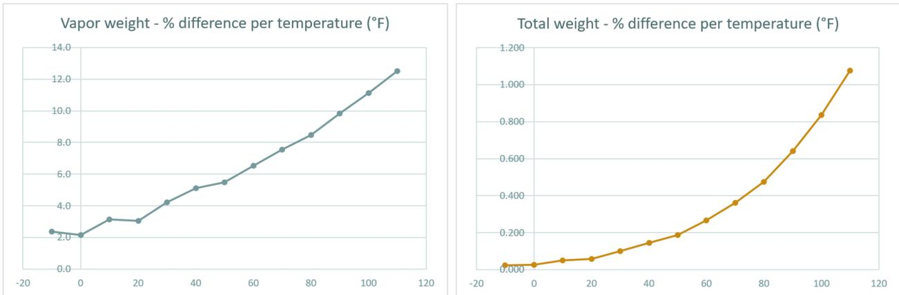
While the total weight deviations are considerably small for temperatures below 60 °F and only exceed the 1 % threshold for temperatures above 100 °F, the vapor weight differences display an almost linear increase from 2 % at low temperatures to 12 % at high temperatures.
