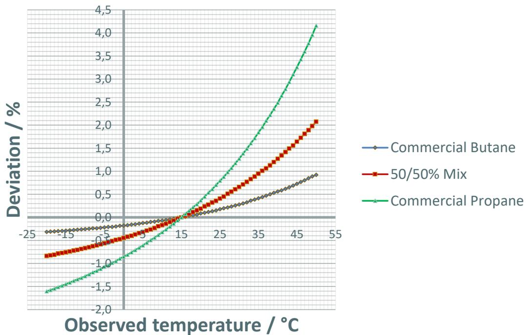
Figure 1: Deviation of CTL values from GPA 8217 / TP-27 results for three products, the base temperature is 15 °C.
