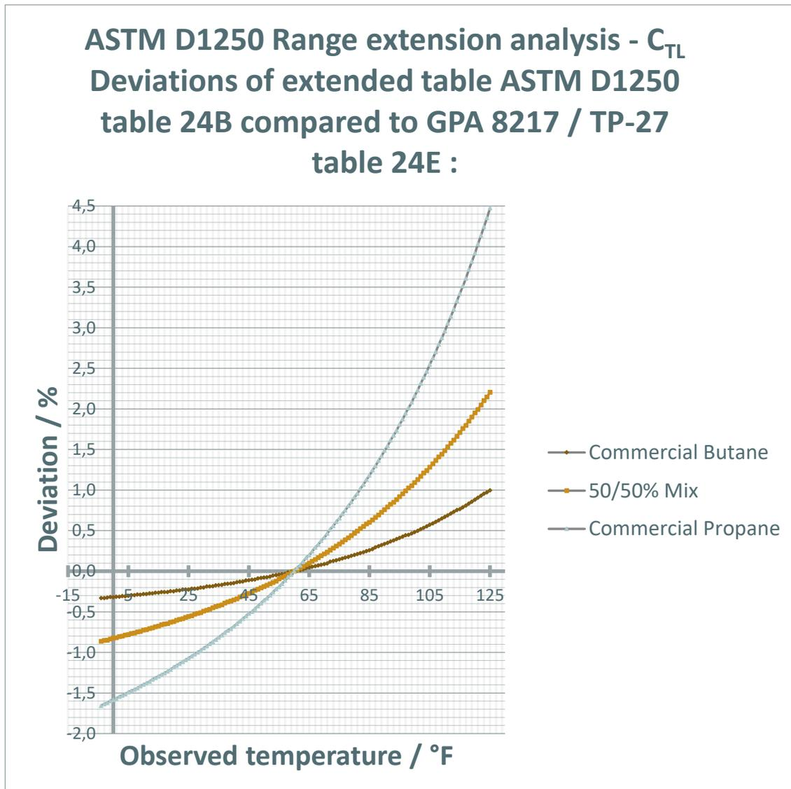
Figure 2: : Deviation of CTL values from GPA 8217 / TP-27 results for three products, the base temperature is 60 °F.
