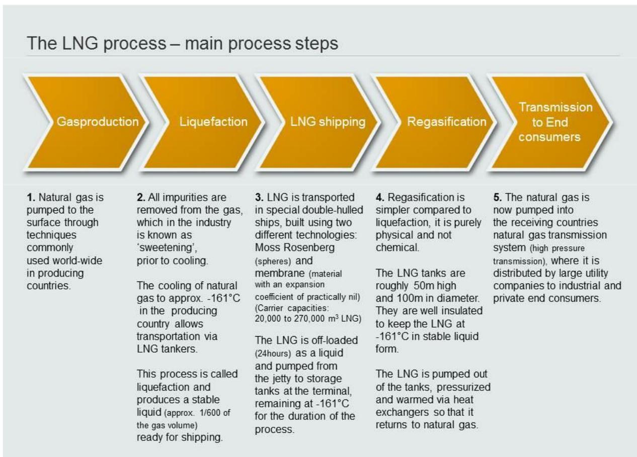
Figure 3: The LNG process – main steps
